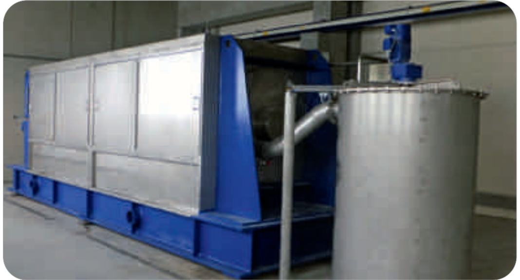
ACAT Screw press 1105 S with mixing reactor Total connected load 11,2 kW
