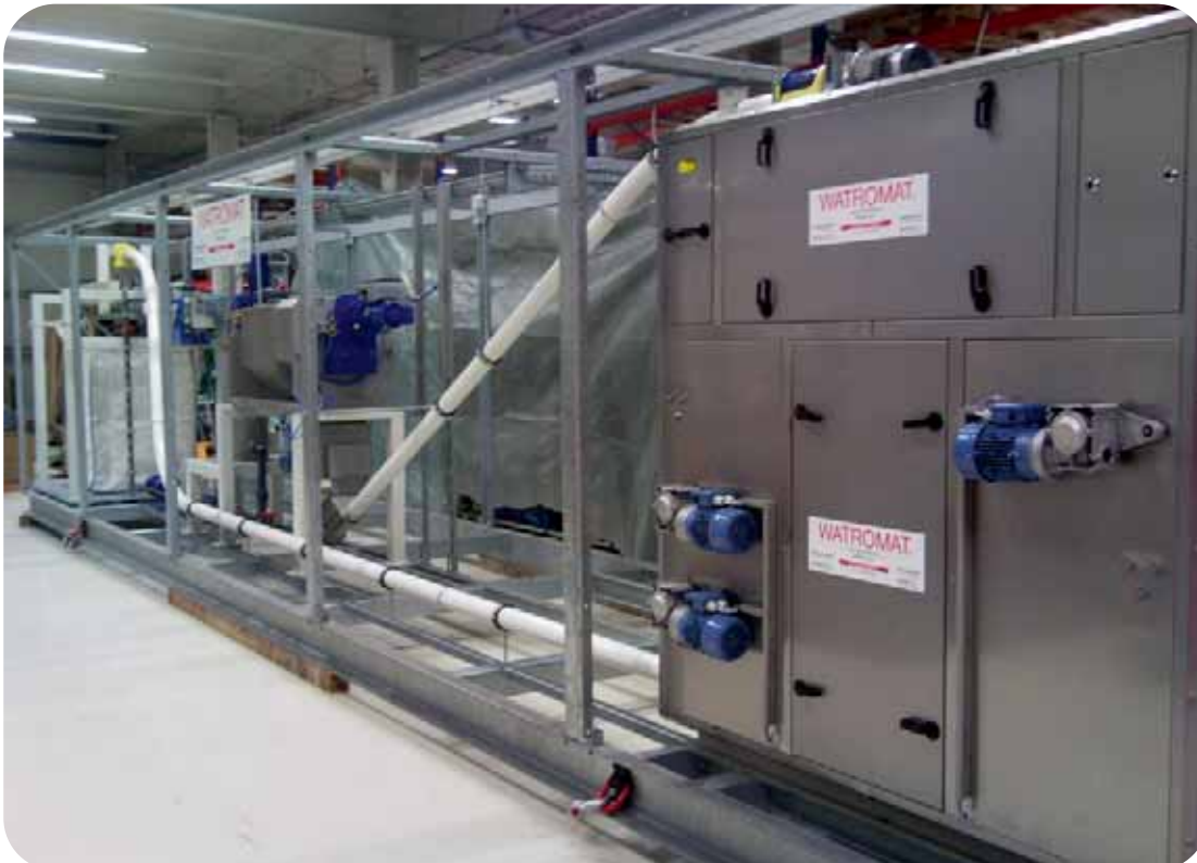
ACAT screw press type AS 250 pre-installed on a Watropur belt dryer
