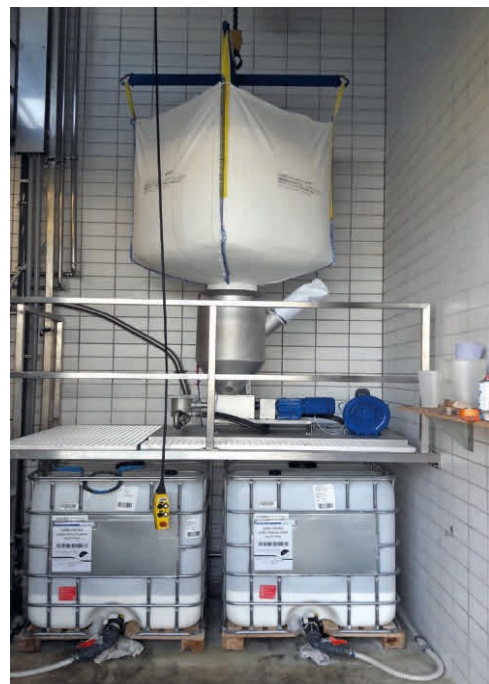
Polymer dissolving unit PPU 3 for sludge dewatering with high-performance decanter
