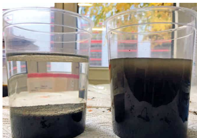
Fig. 2: Sludgy wastewater from a suction vehicle, left picture 3 minutes after treated with FlocStar® Giga 1970 L.
