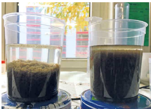
Fig. 1: Wastewater from a clarifier, in the left vessel after treated with FlocStar® Giga 1970 L.
