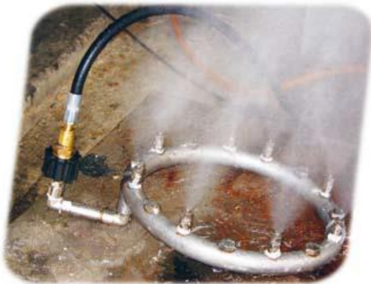
Ring with nozzles spraying Ecosorb® constantly
