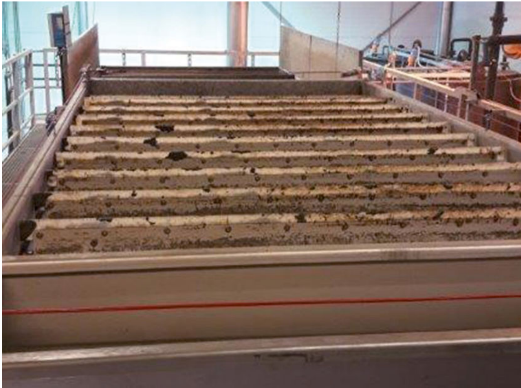
The PET bottles and the containers are shredded. In several further steps the labels and other impurities are separated.
