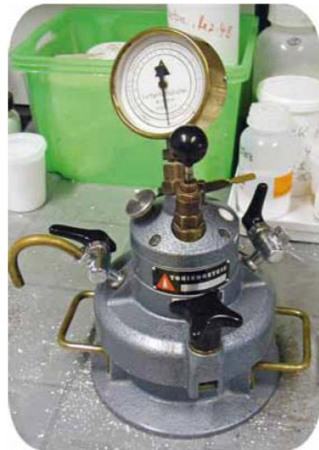
The compressibility of the sample in the instrument is displayed directly on a calibrated scale as the air content of fresh mortar.
