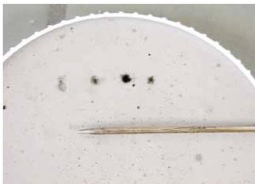
Test Setting Behaviour: Every 5 minutes a needle is pressed into the test specimen
