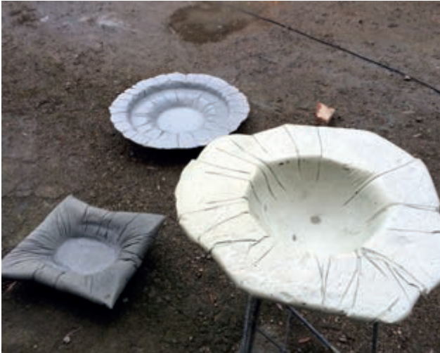
The bowl before (left) and after firing (right) slightly damaged but structurally intact
