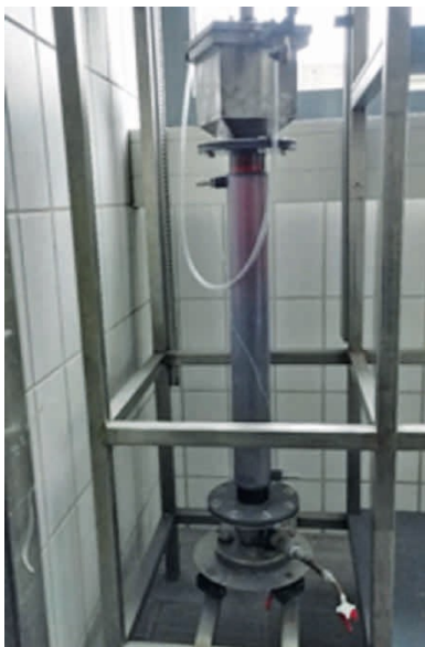
UASB reactor 1 made of plastic
