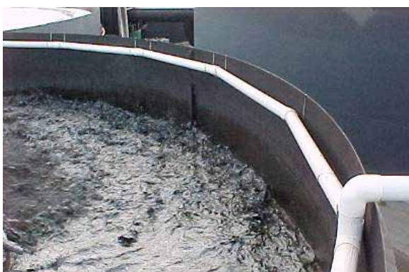
Ecosorb® Vapour Phase Equipment used around a large settling pond.
