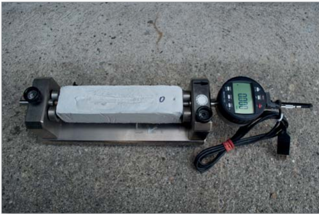
Figure 1: Length determination of the specimen with an electronic dial gauge
