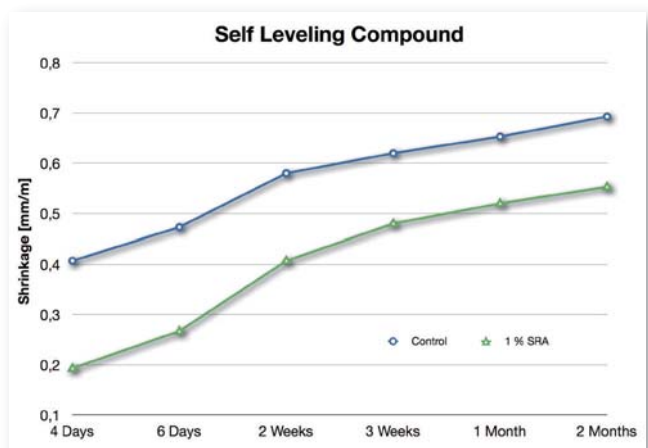
Figure 2: Shrinkage reduction in a self-leveling compound by using a shrinkage reducing agent (SRA)
