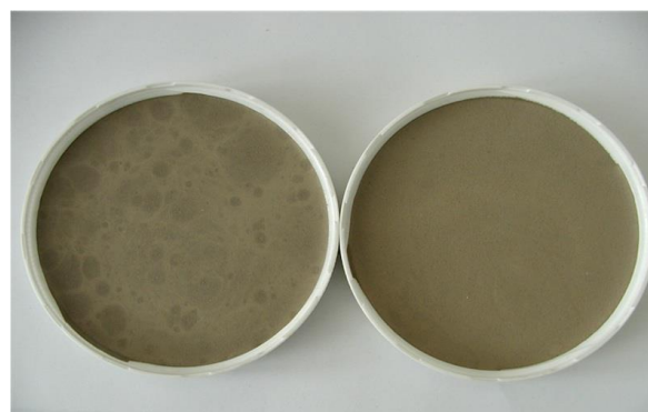
Figure 6: Optical impairment due to wrong defoamer selection
