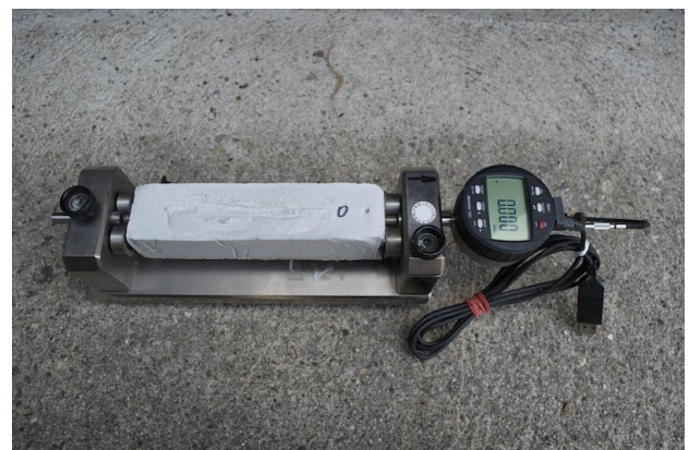
Figure 1: Length determination of the specimen with an electronic dial gauge
