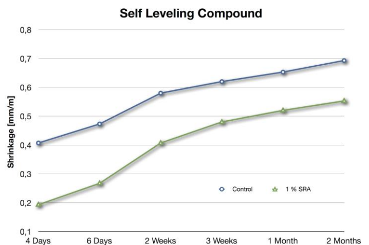
Figure 2: Shrinkage reduction in a self-leveling compound by using a shrinkage reducing agent (SRA)
